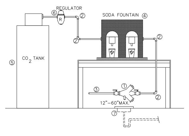
REDUCED PRESSURE PRINCIPLE BACKFLOW PREVENTION ASSEMBLY FOR WATER SUPPLY TO CARBONATED DRINK DISPENSING MACHINE.
